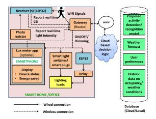
Figure 1: IoT driven smart lighting strategy using proposed HAR model
