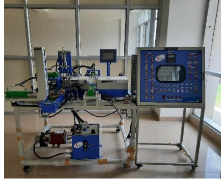
IoT enabled hydraulic sorting mechanism
