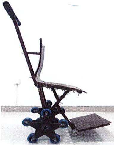
Fully functional Five wheel Stair climber PROTOTYPE
