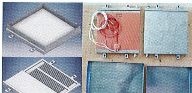
Multi port mini-channel freeze dryer shelf
