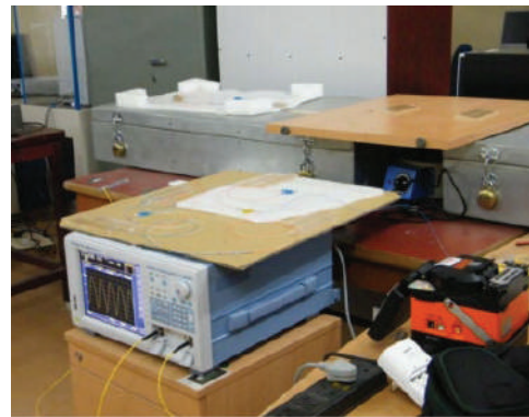
Output fringe pattern measured on OSA of an all-fiber indigenously MZI in the lab
